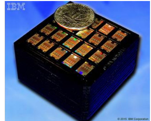
IBM's fully integrated wavelength multiplexed CMOS silicon photonics chip (2015)
