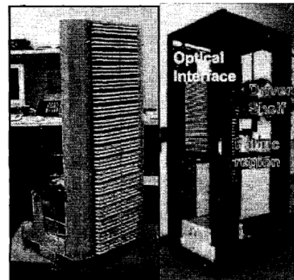
Figure 2. (a) 1296-port optical switch module and (b) 648-port folded-geometry optical crossconnect prototype.
