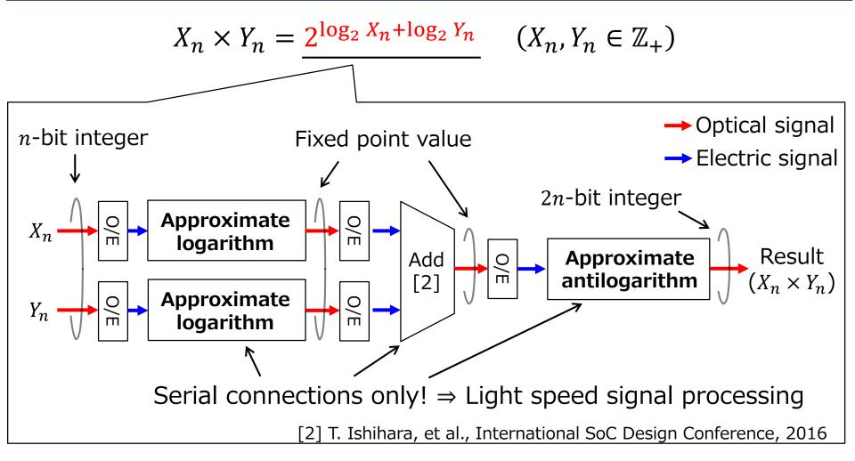
$\checkmark$  Three O/E converters on a critical path for any bit width n
