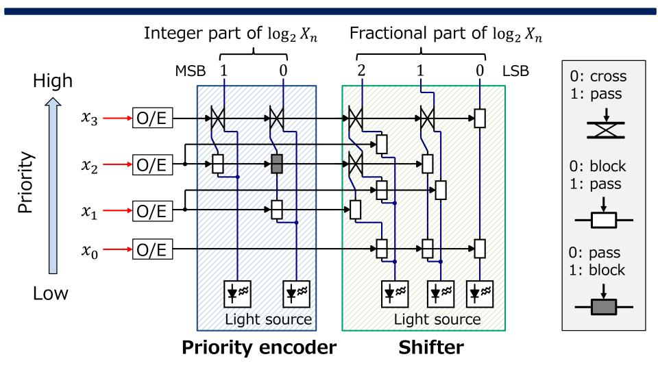
✓ Only one O/E converter on a critical path for any bit width n
